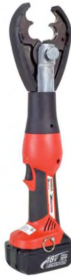
CMB1 Cuts 4/0 ACSR CMB2 Cuts 477MCM ACSR CMB3 Cuts 3/8" guy wire
